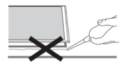
**NOTE //** Do not use any joint sealant. The appliance's sealing strip ensures a sufficient seal between the appliance and the benchtop.
