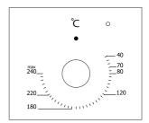
**Program Button:** Helps to set with which heaters the food placed in oven will be cooked. Heater program types in this button and their functions are stated below. Every model might not have all heater types and thus program types of these heaters.
