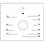
\*Mechanical Timer Button: Helps to set time for the food to be cooked in the oven. Timer de-energizes the heaters when set time expires and warns you by ringing. See cooking table for cooking times.
