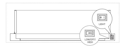
**IMPORTANT:** To operate the unit, ensure that the power is turned on and the front visor is fully extended. This will provide access to the light and speed controls.
